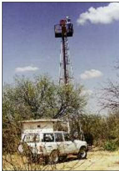
Water level recorder near Stampriet high above ground measuring the artesian water level
